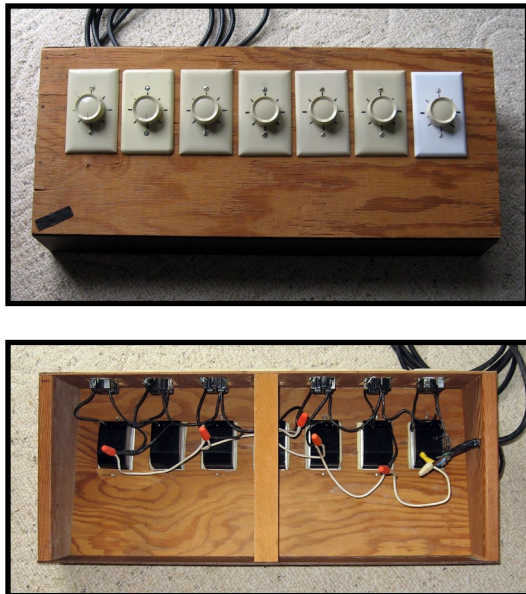
Figure 1.3 — Two views of a home-made lighting control board.
